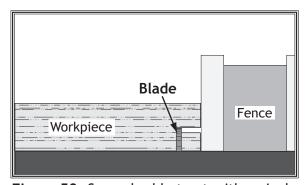
**Figure 58.** Second rabbet cut with a single blade.
